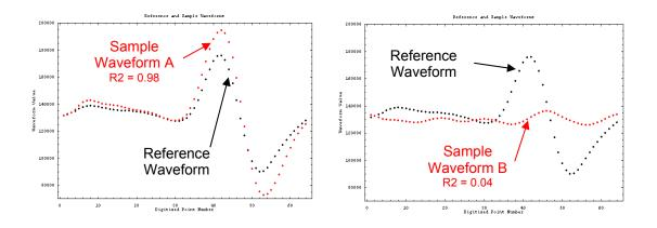
An accepted mathematical procedure to compare curves or numeric arrays is the **Linear Least Squares Regression** analysis. This analysis results in a measure of the similarity ( $\mathbf{R}^2$ ), between the waveform of the **sample** gas and that of the **reference** cell gas. A perfect similarity would give a value for  $\mathbf{R}^2$  of 1.0, and a total mismatch would be 0.0.
