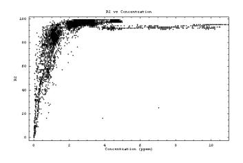
With lower levels of sample gas, the  $\mathbf{R}^2$ s decrease, and equal zero when there is no gas present. As the signal from the gas becomes stronger, the effect of noise, both electronic and optical, is reduced and the  $\mathbf{R}^2$ s will increase (i.e., the signal to noise ratio will increase). The general shape of the plot is the same for all gases, however, the x-axis values will depend on the sensitivity of the instrument to the gas species being observed.
