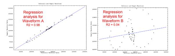
The blue line represents the **Linear Least Squares** fit of the data and is the best fit of a straight line between the reference (X) and sample (Y) data points. The slope is a component in the ratio-metric calculation of gas concentration.
